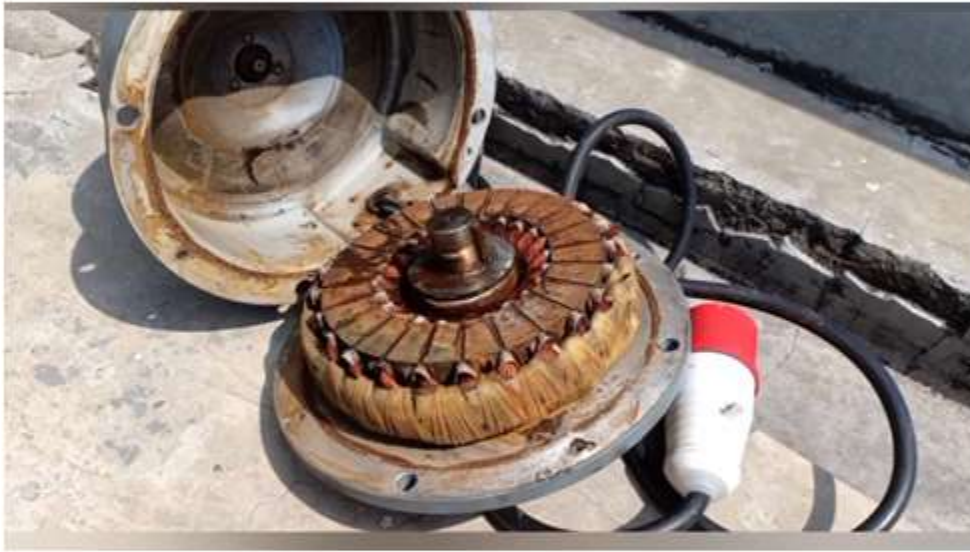
Repair Motor Gondola part1
